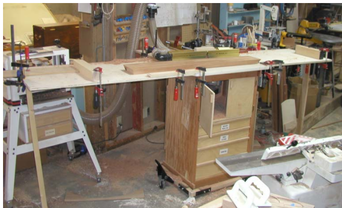
A ten-foot router table from the scrap barrel
