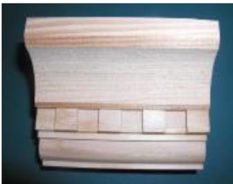
are matching, is to make several pieces of different designs, perhaps a couple feet long. Cut an inch off of each piece. Then lay them flat on the table on the end grain and start moving them around like a puzzle. You will easily be able to see the profile and can settle in on one you like. You'll
