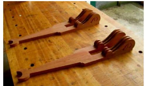
The "bones" also need three half-circle bent laminations for the three arches; we made the forms, bent the laminations, and threw away the forms as soon as we could bring ourselves to part with such carefully-made items. Torsion
