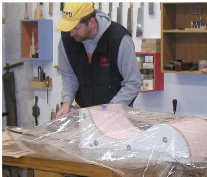
glue--up of three laminations, installing it in the vacuum system and pumping it down. Looks easy, well actually it doesn't, when you've been there before.
