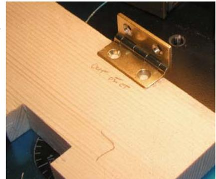
**Test cut on the flip side of the jig**
