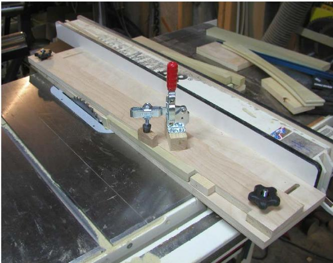
The tapered leg, on the second cut, needed to be elevated to assure that the exit cut was perpendicular across the leg. BLAM (again), shoot a little spacer block in place for the second set of cuts. Then rip it off and recycle it.
