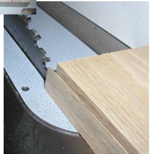
the top of the board is just flush (plus or minus). Trial and error here will produce the part you need. If you're flush or a little less than proud on the cut, you will have a feather of an edge for your wedge. It may not even be perfectly straight, but brother, is it fine.
