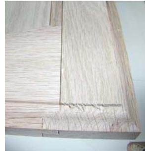
Cut a v-e-r-y thin wedge and glue it in the crack. How to cut it? Tilt your table saw to about two degrees. I experimented with steeper angles and got wedges, not filler shims.
