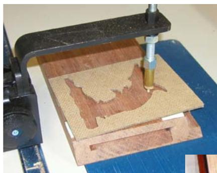
To use it you make a template like the dolphin pictured. Double tape the template to the top side of your work and route the bottom, tracing the pattern on the top.
