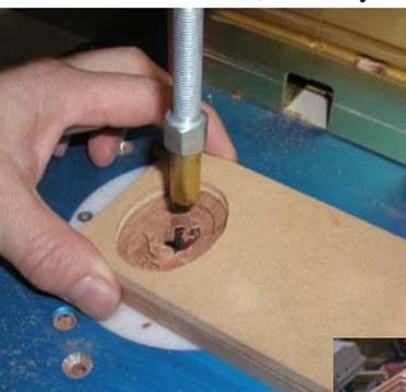
Suitably registered, the back was routed first, half way through the frame, about 1/8" to form a rabbet. Then the fronts were routed. A loose piece in the center dropped away, usually tossed conveniently onto the floor by the 1/8" bit. The pin router made a difficult production job very easy.
