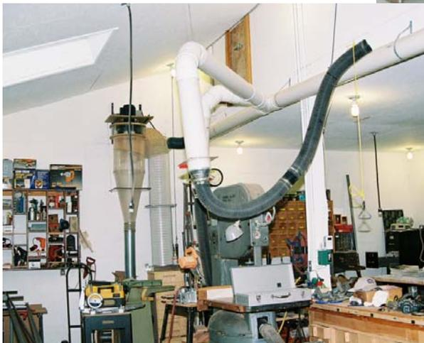
lathe, large sanders, router table, band saw, jointer and planer. The 6-inch pipe is reduced to 4 inch at the machine. Dust collection is two fold at the router, cabinet saw and band saw with collection at the top and bottom of the machine. It is really nice to be able to cut wood on the cabinet saw without having saw dust blow back at you from the saw blade. And, it is safer to have a guard with dust collection.
