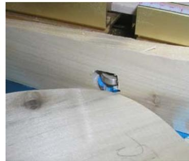
A zero clearance fence was the 'obvious' answer. A scroll saw quickly made a clearance hole for the bearing. Cutting the zero clearance is a bit tricky. Holding it from moving sideways and stopping at the correct depth were simultaneous challenges
