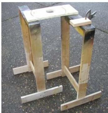
I used this style all summer, 2007, in building the stagecoach (see issues June-Sep 2007). So I made a couple and they have been used a lot more than any other horse. They are essentially a configurable work table. Clamp things to it for assembly or modification.
