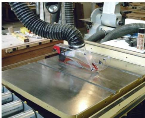
Another problem, the sawdust was terrible. I had a dust collector that removed the dust from the bottom of the saw. But, the dust generated on the table top, when cutting a board, was bad. I needed a better way.
