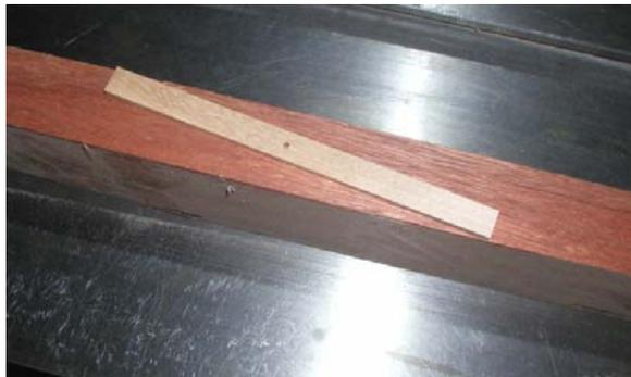
ter represents the board's middle. This device could be moved along one axis of a board, allowing the user to locate the middle anywhere he or she wishes.
