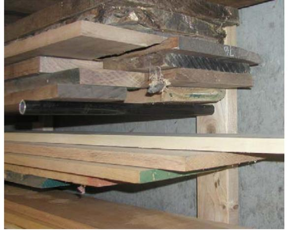
rack will hold 10-foot lumber easily. The five 8-foot vertical supports have pipes spaced 12 inches apart, so that's 30 pipes to cut. If you have access to a metal cutting bandsaw you're in fat city.
