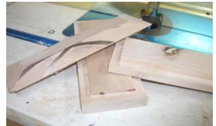
Version 3) Beveled first at 23° and not as deep. Then rabbet the back side all the way around. Perfect, except that the rabbet is only needed on the sides, not across the top and bottom. Salvage this set with some glued in filler strips across the top and bottom.
