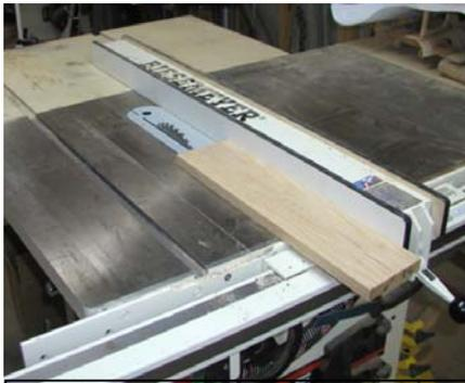
**Figure x. A Safe Configuration.**
