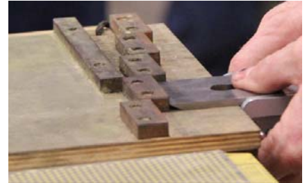
Set the micro bevel angle (30)
