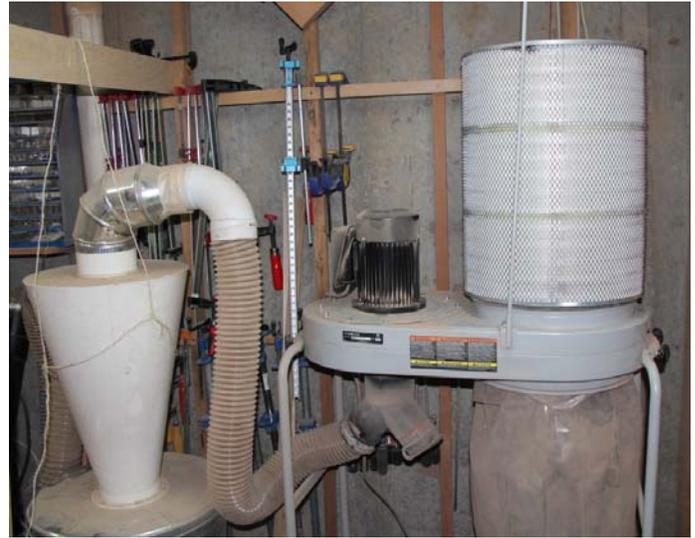
the rigid shape, according to the manufacturer, is easy to clean by pushing compressed air through the canister while mounted on the machine. Limit pressure to 60 psi to avoid damage to the filter. The dust falls into the plastic collection bag.
