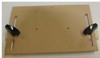
The base is 1/4" hardboard or plywood. It could be thicker and you'll just lose a little routing range on the bit. This one is 12 x 10 inches. Just be sure in planning your own size to make the jig wide enough
