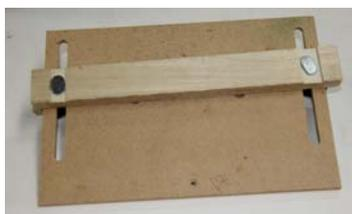
The fence is roughly 1x2" with two holes for bolts. This one has a table saw dado to provide for the heads of the T-bolts, cut with a standard 1/8" saw blade making several quick passes sideways.
