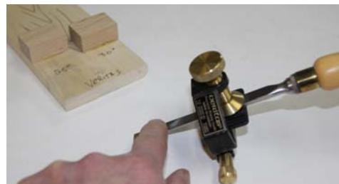
To test this new jig, I went through one set of chisels. The first chisel, ironically the only one, was way off on angle. It was obvious that it had seen a hand-held sandpaper belt method some time ago. It took about 10 minutes alternating between 150 and 220-grit sandpaper to get it flat and back to 25°, finishing up with wet stones at 800, 4000 and 8000. Wow, does it cut now!! Fortunately all the other chisels took less than two minutes each to run through the grits.
