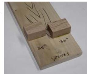
We use a jig to hold the chisel at a consistent angle, but how do you set that angle? There are several
