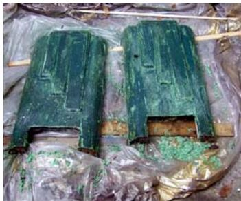
I stripped the main castings with Citristrip. It took many applications over several days, followed by an angle grinder with a wire cup to take it down to bare metal. Next time I will pay someone to sand-blast it for me. The smaller parts I stripped with a wire
