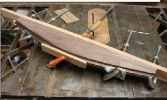
clamped on an end cap form to cool and dry for a few hours. The cooled spacer was then glued, screwed and clamped to the chest lid end cap.
