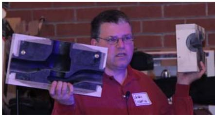
Metal is poured into openings in the block, gases and air escape from the trapped areas through vents in the mold. When it cools, the mold is broken away from the part. The mold is only used once, so each part must have a mold created. The pattern must be durable enough to be used thousands of times.
