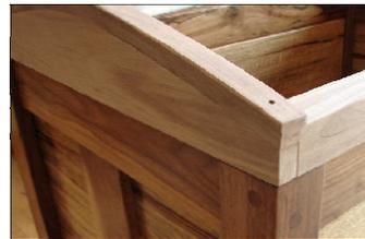
The screw hole on the cap cover was filled with a hand carved plug, cut flush and sanded.
