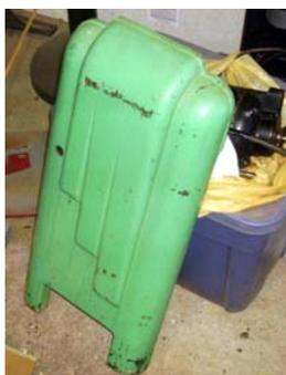
And one of the cast iron Art Deco stand ends, with the motor behind it:
