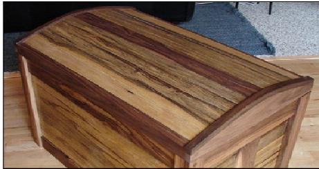
The chest lid project starts with the end caps which capture 12 staves. The end caps are assembled from three parts: A band sawn base, steam bent spacers and covers to create a slot for the staves. The slot can also be cut with a router which would be much faster but not nearly as interesting either from a build or esthetics perspective.
