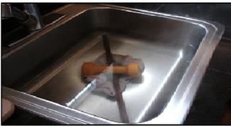
water brought to a boil on the stove. Soaked for 20 minutes, the spacer was
