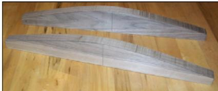
The one inch wide base of the end caps were cut on a band saw and cleaned up with a few sander passes.
