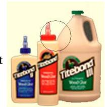
**Temperature** is the single cause of failure in a glue joint. Refer to the label on the bottle. Have your glue, wood and air temperature five degrees above the minimum. Under clamp pressure, water is forced out and absorbed into the wood. The polymers need enough mobility to combine and cure. If the temperature is too low, they can’t do that and it forms a chalky joint with no strength. Storage and transport at low temperatures is ok, even up to five freeze/thaw cycles.
