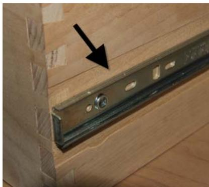
But, you can make a drawer narrower. A little bit. The mounting screws still have to not poke through.
