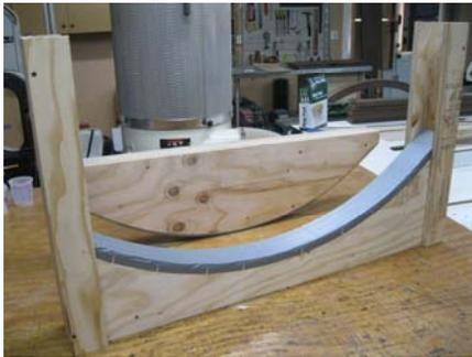
A couple of 'U' shaped channels on each end of the forms would help align each slat as it was put into the form, and lend stability during clamping. After the clamps are all in place, those channels are easily removed to keep from being glued in place by the squeeze-out. A couple of screws held them and allowed quick and easy removal while the glue cured. Satisfied the bending form was ready, it was time to start cutting slats.
