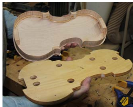
The mold is removed!
