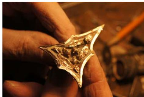
After cooling, crack the mold, pick away the pieces, fine tune the casting with small grinding tools and it's ready for inlay. A little epoxy and a press fit into the wooden receptacle completes the process. Outstanding and totally unique! Thank you, Chuck.
