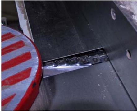
The old cutter came out and the new one dropped in, two bolts. Installation instructions said to use newspaper for shim stock if needed. Testing the height on each end of the assembly against the out feed table made me want to shim one side, a couple thousandths. One sheet—perfect.
