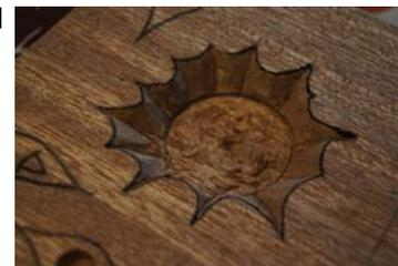
ving slopes the edges down to the bottom of the drill hole. Not a critical job because it's going to become the bottom of the casting.
