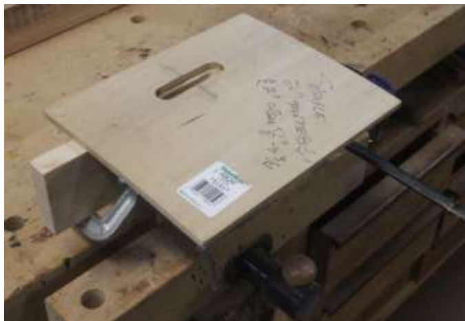
Jig in the vise, ready for routing.
