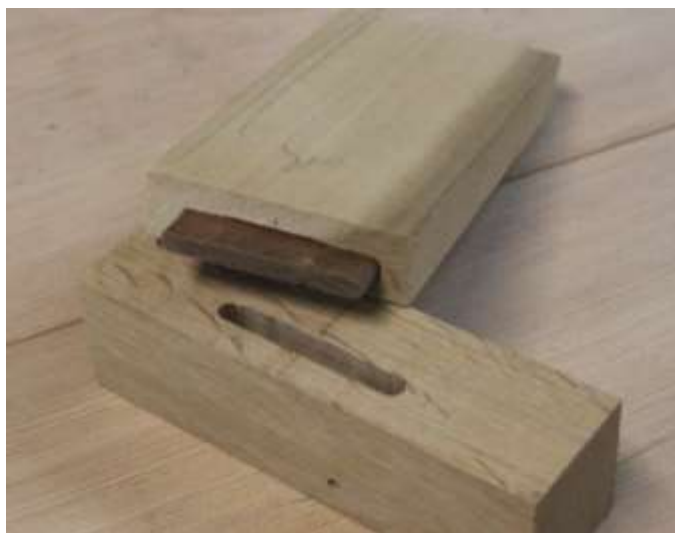
Mortises cut. Tenon stock in place, ready to glue.
