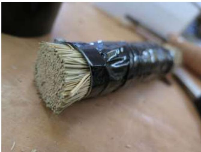
Making polissoirs (a wood polishing tool) from local materials during a woodworking class is always fun, though it isn't always easy. Getting the broom corn for the core of the tool is usually a snap. Hose clamps we can usually scare up. But then we need wax and something to wrap everything up tightly.
