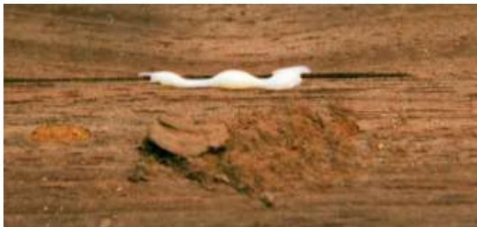
sanding sawdust from a nearby pile into the glue and massage it into the crack. Leave it to dry. I've tried pre-
