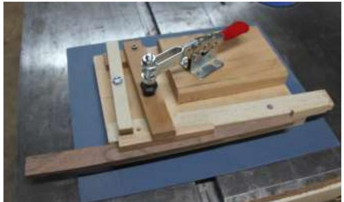
Safe to use, it's a rip on the table saw. Little finger hooked over the rip fence, firm grip on the clamp. If they were a little longer, the offcut could be chopsticks.
