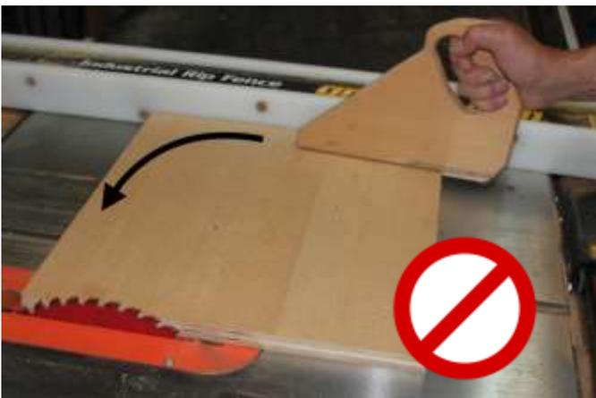
*Pushing close to the fence twists the board towards the back of the blade. EXTREME DANGER.*
